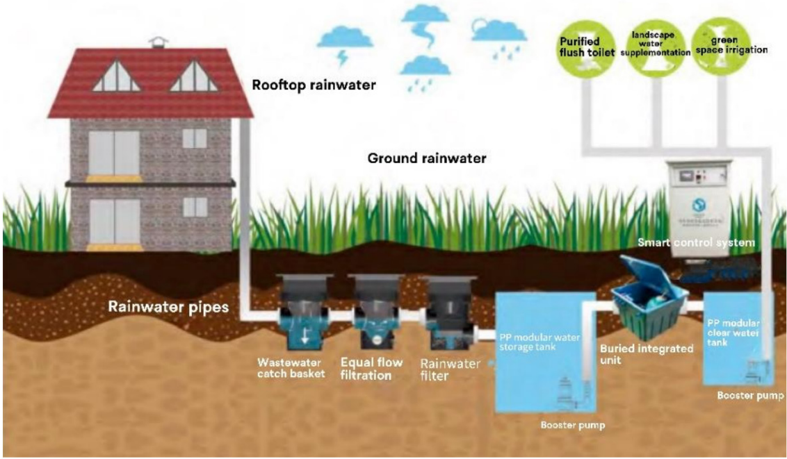
Fig. 1 Rainwater Recovery System [3]
